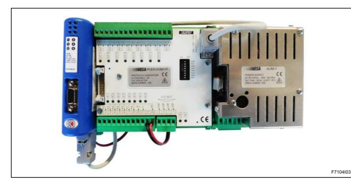
ESA PLEX-COM1 is a serial protocol converter used to suervise the ESA ESTRO flame control device or ESA REFLAM flame presence indicators. The card allows any control or supervising comand (PLC, PC, DCS etc...) to comand and receive information on the burner state via the Modbus RT serial protocol in a quick and versatile manner.
